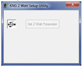
2. Connect the KNG-S Portable radio to the computer with a USB cable and turn the radio on. The display will change when the utility recognizes the radio connection.
