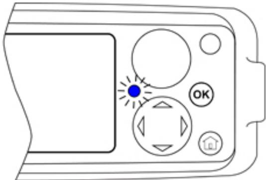
5. While holding the push-to-talk on the microphone connected to the remote control head, turn on radio power. (Note: The radio must be connected to the computer before power-up.)
